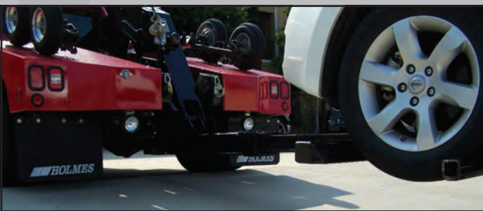
The optional power tilt operates through a 30-degree arc, providing positive tilt for increased vehicle clearance and negative tilt for ease when hooking up on a slope.
