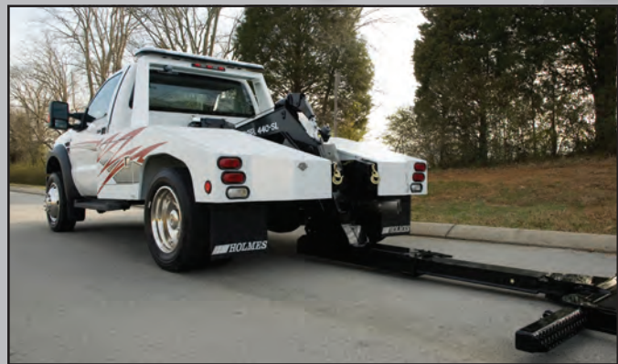
The low-profile body design provides superior visibility and 73" of reach, so hooking up to most vehicles is quick and easy.
