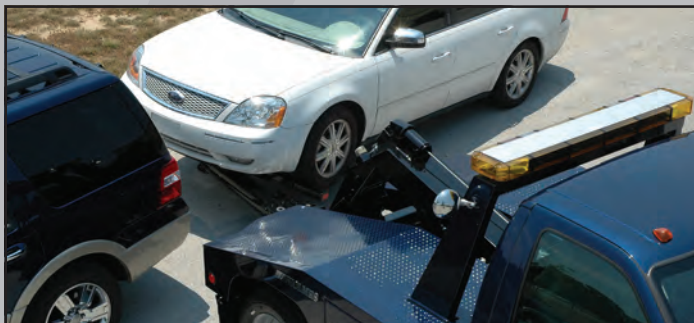
The Holmes 440-SL is capable of hooking up to a vehicle at a 90° angle such as parallel parked vehicles.
