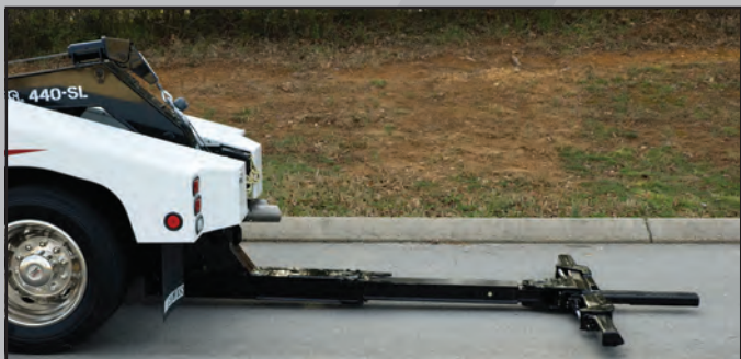
The low-profile body design provides superior visibility and 73" of reach, so hooking up to most vehicles is quick and easy.
